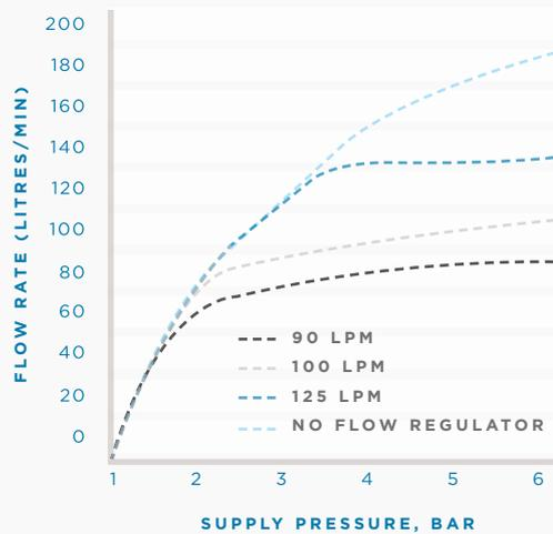
Easyflush Direct requires a minimum flow rate of 90 litres per minute (typically 22m pipework) and is therefore not generally suitable for domestic installations.
