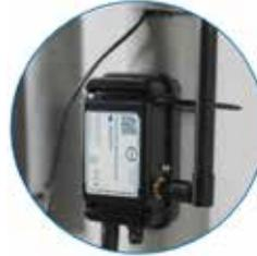
TMUs take temperature samples every 10 seconds (for hot, cold or blended supplies) and automatically begin recording additional data when outlet usage is detected.
