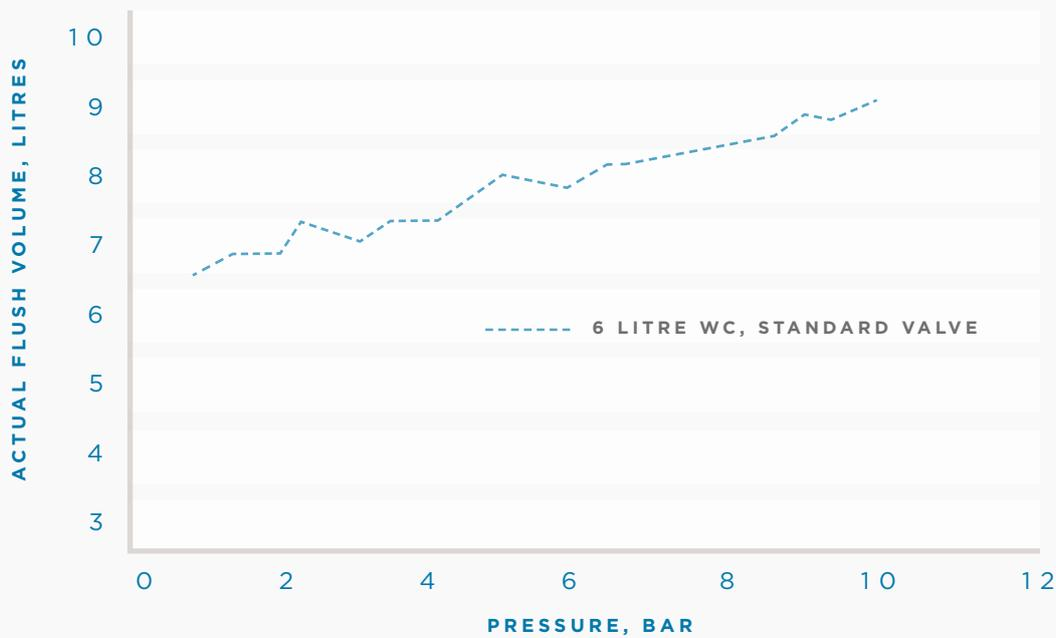
Installing a Cistermiser Easyflush can save up to 84,000 litres per year as shown below:
