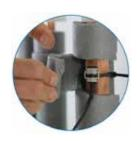
Each TMU accepts up to 4 temperature probes (configured as 2 pairs) which simply affix to pipe work surfaces using clips (15mm) or cable-ties (>15mm).
