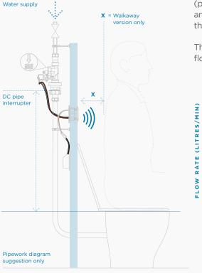
The flow rate can also be reduced by turning the adjuster screw in the middle of the valve (clockwise to reduce flow) or by fitting a third party pressure reducing valve above Easyflush Direct.
