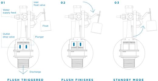
Water pressure lifts plunger, opening outlet drop valve and holding inlet float valve in the closed position.
