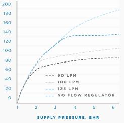
Easyflush Direct requires a minimum flow rate of 90 litres per minute (typically 22m pipework) and is therefore not generally suitable for domestic installations.
