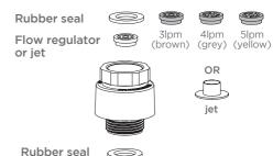
In some circumstances a squeak may be heard when the valve closes. If so, the DC pipe interrupter jet may be used to reduce this.
