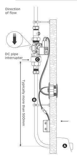
The DC pipe interrupter is supplied with 3 flow regulators. Select the appropriate flow rate to match the sparge (A) and the volume of the pipe (B) to prevent overflow from the DC pipe interrupter (C)
