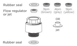
In some circumstances a squeak may be heard when the valve closes. If so, the DC pipe interrupter jet may be used to reduce this.
