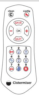
most effective when the © clean button is held down as the ICU is brought close to the sensor. It can take up to 3 seconds for the product to sense the ICU.
